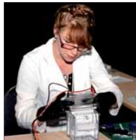
Natalie Donaher prepares the electrophoresis chamber to run the extracted plant proteins on a PAGE gel.
